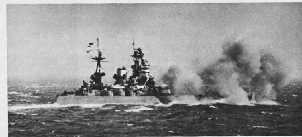
H.M.S. Nelson has all three turrets forward on long foredeck, is cut off sharply abaft her mainmast. Nelson and Rodney mount 16-in. guns, are still the most powerful British BB's.
